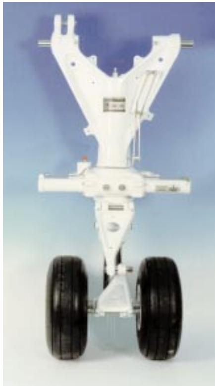
Designing better landing gear faster — that's the aim of the Liebherr-Aerospace engineering team as they exercise conceptual ADAMS models in simulation. These conceptual tests provide the early insight needed to minimize problems later in detailed design. The result can be top-quality finished products like this nose gear, which Liebherr-Aerospace supplies for the Embraer Regional Jet 145.
